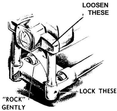
If horizontal alignment of shafts is not within 1/16", loosen the two set screws in the tool base which lock it to the twin tubes and "rock" the tool slightly on the tubes. There will be sufficient lateral movement by gently rocking to achieve alignment.
