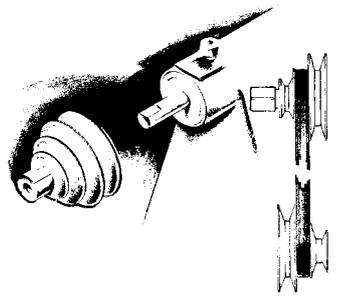
Remove pulley guard from SHOPS MITH and replace headstock pulley with special pulley supplied in Adapter package. Be sure alignment of headstock pulley, in relation to motor pulley, is correct.
