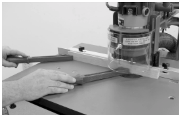
Figure 28. Straight-line routing using a push stick.
