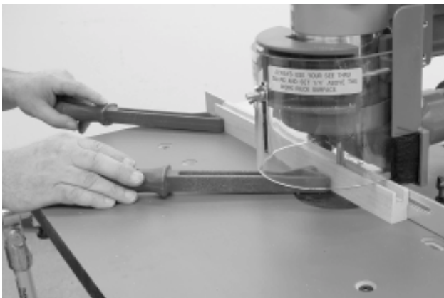
Figure 31. Cutting a groove with the grain by guiding it against the Overarm Router Fence.
