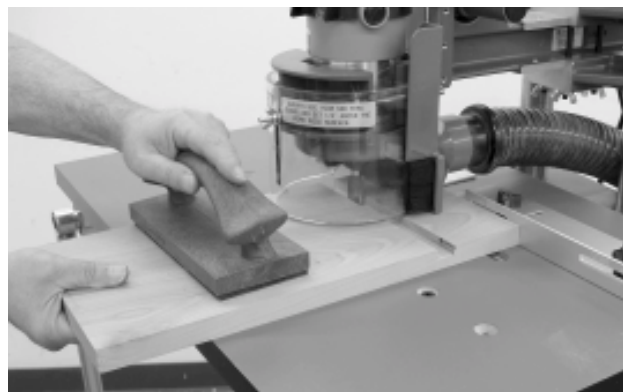
Figure 29. Cross-grain routing using a push block.
