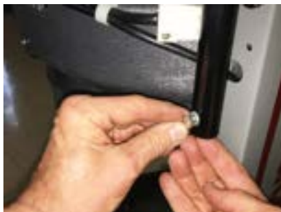
Figure 10: Tighten Rear Handle & Spacer securely into the Leg with Hex Bolt.
