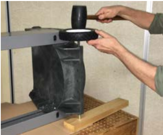
Figure 6: With the housing on its side, position the base pan so the straight side faces towards the front.
