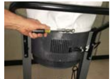
Figure 12: Tighten the Clamp & Rack between the two ribs on the top of the Main Housing.
