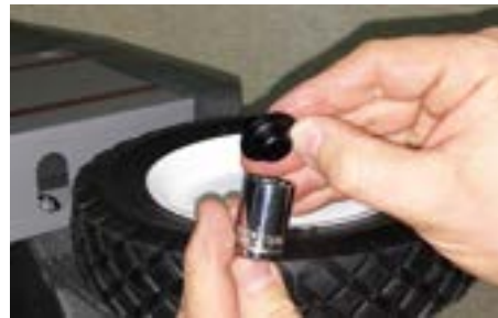
Figure 7: Place the Wheel Retainer inside a 9/16" socket.
