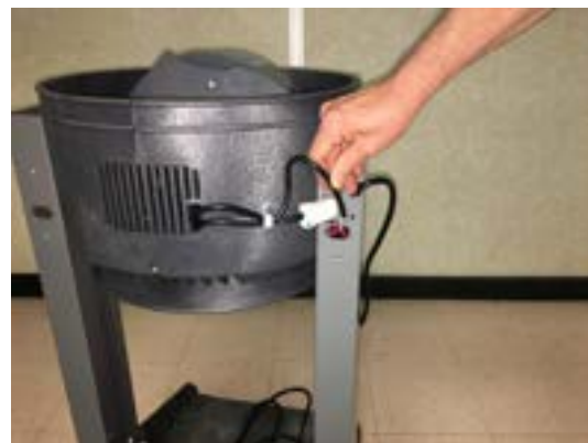
Figure 15: Feed the second black wire with two leads through the hole near the plug.
