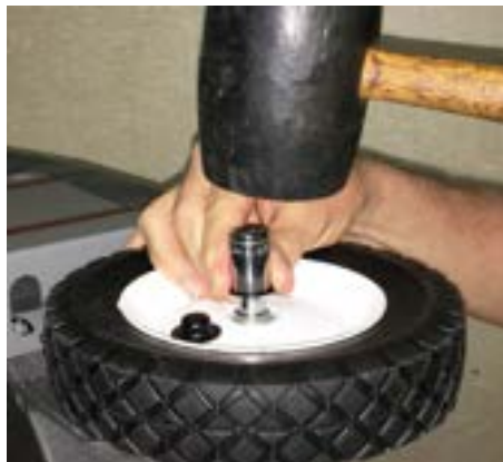
Figure 8: Drive Wheel Retainer on to the Wheel Shaft with a mallet.
