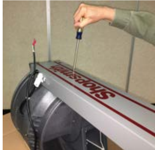
Figure 5: Support the left leg as you attach it to the Main Housing. The narrower side faces toward the front (3-hose inlet) side.
