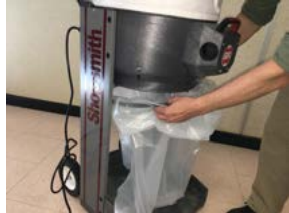
Figure 13: With Bag Retention Strap in place, slide collection bag over the lower rib on the Main Housing.
