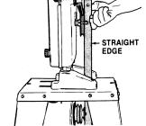
Figure 1 - Use a straightedge to align the pulleys.
