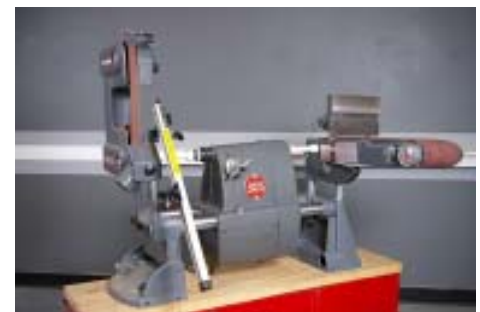
Belt Sander & Strip Sander on three Storage Cabinets
