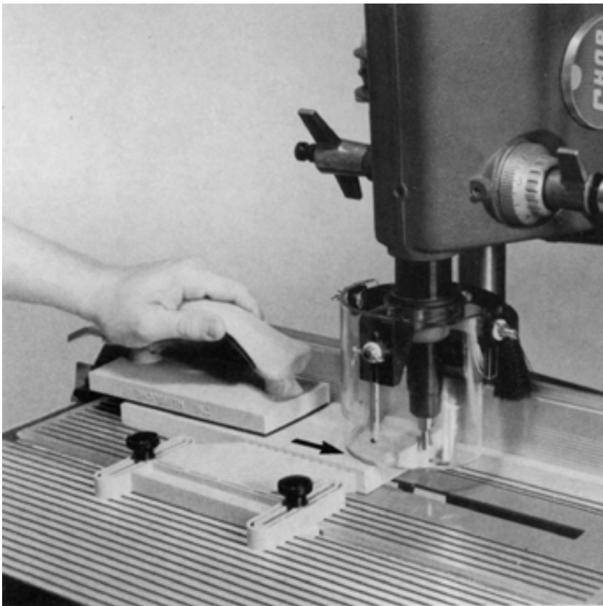
Figure 10-12. Make dovetail slots using a feather board and push block.
