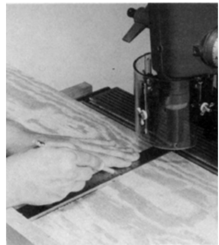
Figure 10-17. Two passes are needed on an extra-wide workpiece. Be sure to align the bith with the kerf.
