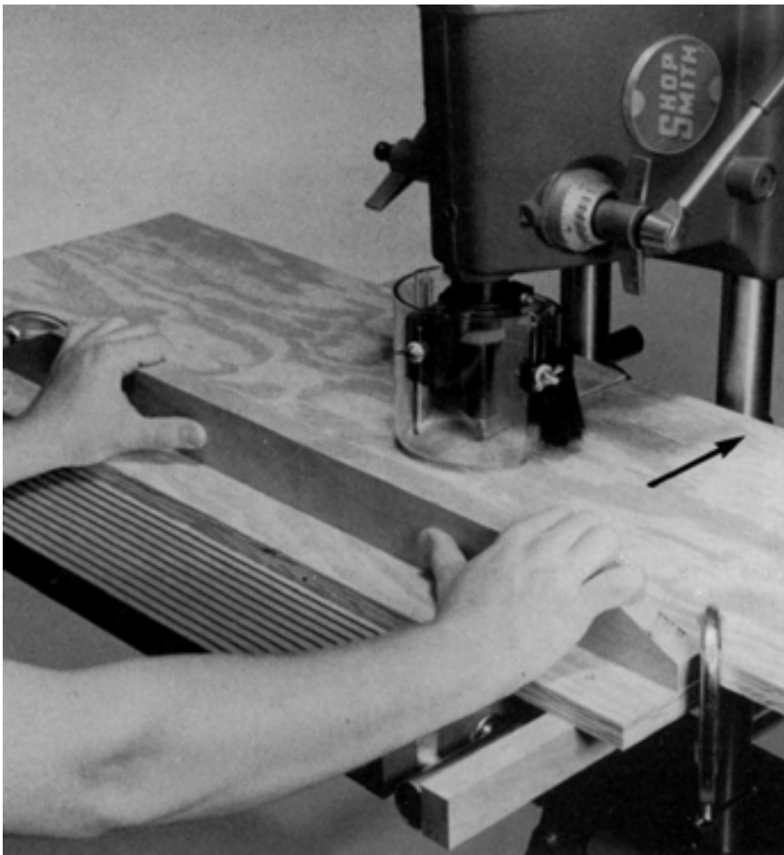
Figure 10-15. A sliding table greatly simplifies cutting a dovetail slot in an extrawide piece.
